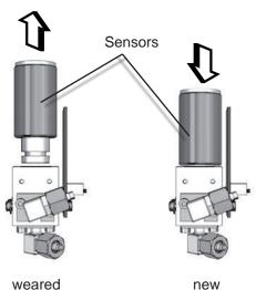
Now re-assemble the sensor unit in reverse order, but do not yet install it into the analyzer as it requires a signal adjustment.
